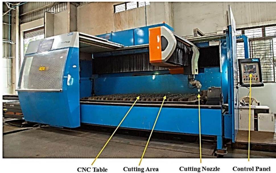
Fig. 1. Experimental set up of laser cutting process
