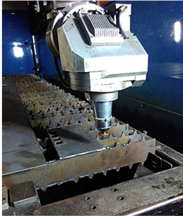
Fig. 1. The laser cutting process of Hastelloy C-276 sheet
