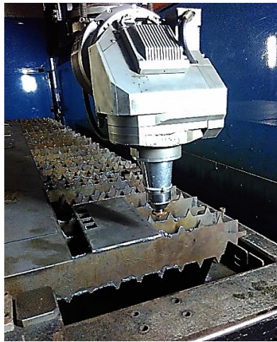
Fig.1. Laser cutting process of Hastelloy C-276 sheet
